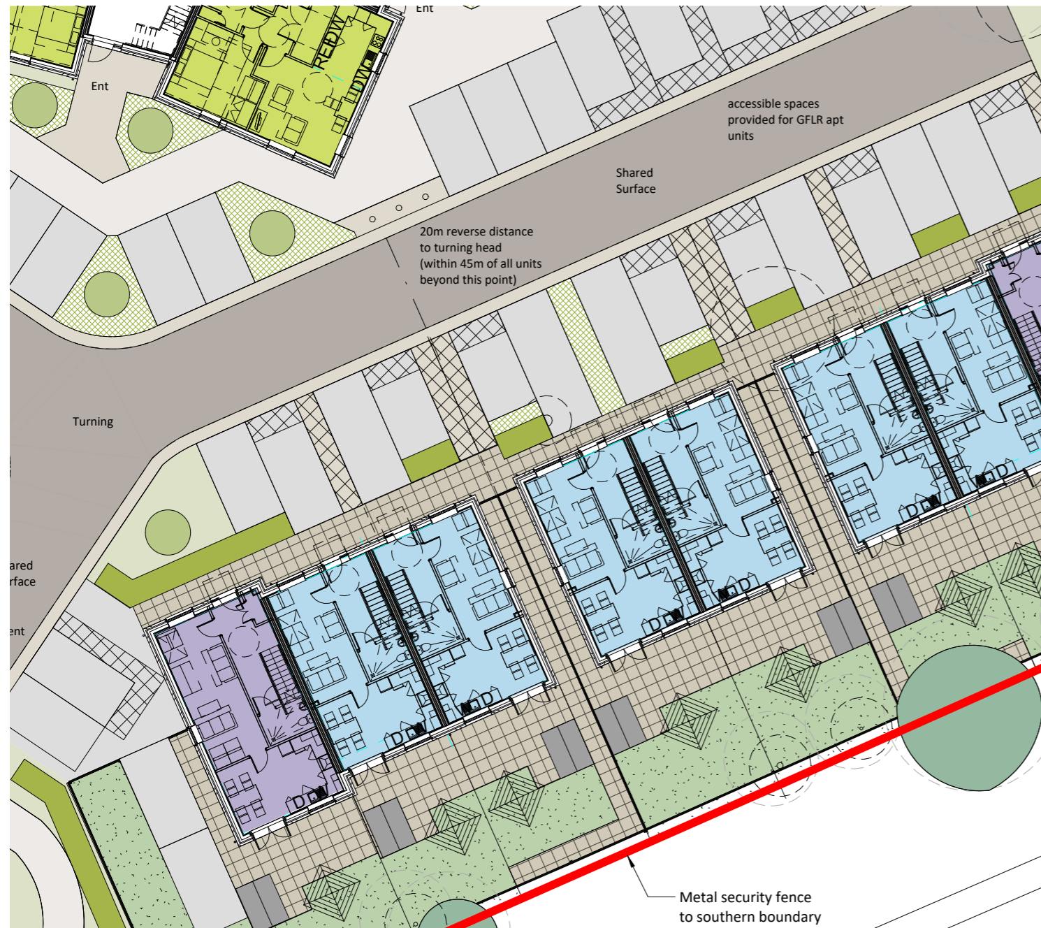
Site plan extract showing open frontages and surveillance of the street with secure rear gardens
